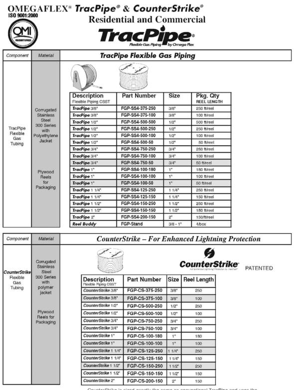
CounterStrike is sized exactly the same as conventional TracPipe and uses the same AutoFlare fittings.
