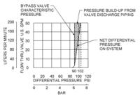
pressure in the system will rise under bypass conditions, as illustrated on the curve.
